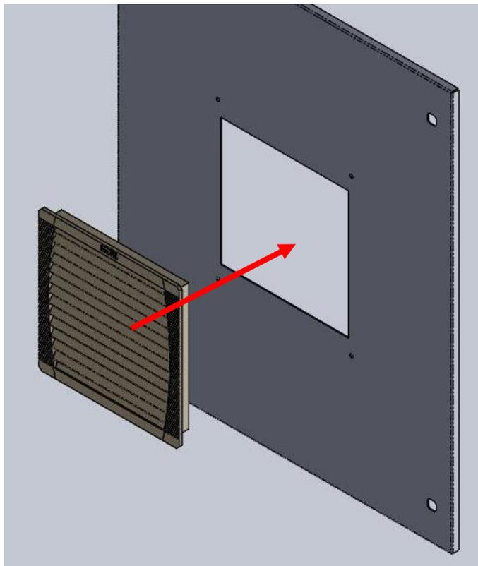
2. Remove Rain hood frame and spray deflector from packaging and remove plastic plug to separate the two pieces. Plastic plug can be discarded. Using frame piece, mark and drill (4x) 1/4" holes around filter fan in enclosure wall. Refer to drill detail on next page. Install frame piece and spray deflector on outside enclosure as shown. Sealing washers and lock-nuts to be on inside of enclosure wall. See assembled view on next page.
