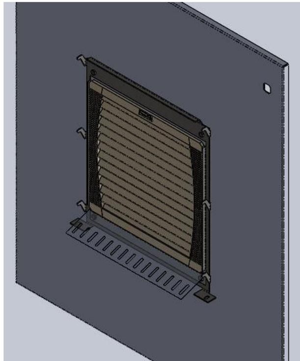
Assembled Frame with Spray Deflector (deflector transparent for clarity)
