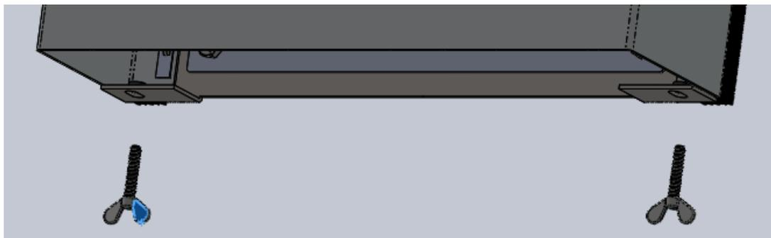
Tool-less wing screw fasteners (Standard)
