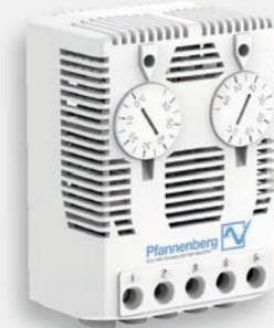
Filterfans 4.0™ can be optionally equipped with Pfannenberg FLZ Series thermostats and hygrosats, allowing for operation only when cooling is actually necessary. This allows for additional energy savings, reduced maintenance and extended service life.
