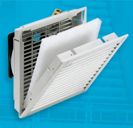
The 3rd generation Pfannenberger Filterfan® saw another improvement in performance and efficiency. This was a precursor to today's fin design. For the first time, a patented folding mechanism allowed for the replacement of two different sized filter mats, in just a matter of seconds.
