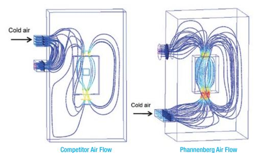
As the diagram shows, Pfannenberg's approach to internal airflow paths supports both natural convection and provides cool air where needed - below key electronic components. Natural convection states that hot air rises, creating a natural airflow inside the enclosure. All of our Cooling Units pull hot air from the top of the enclosure and with the longest distance possible, pump the cool air to the bottom of the enclosure, helping eliminate "hot spots" inside the cabinet.
