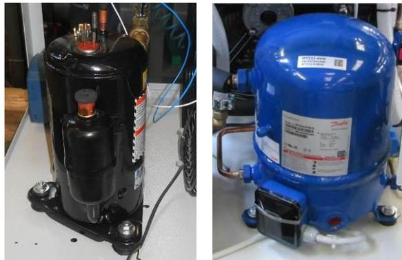
Picture 17– Compressor placement for CCE 6101 – 6201 – 6301
