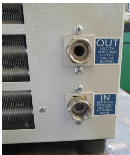
Picture 3 –Hydraulic connection plate
