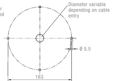
Two different drilling templates are available for fixing the light (direct mounting). M5x 8 threaded bushes are set into the base of the light for fixing according to drilling template 1. Drilling template 2 allows the light to be fixed using 4 through bolts or similar from above.
