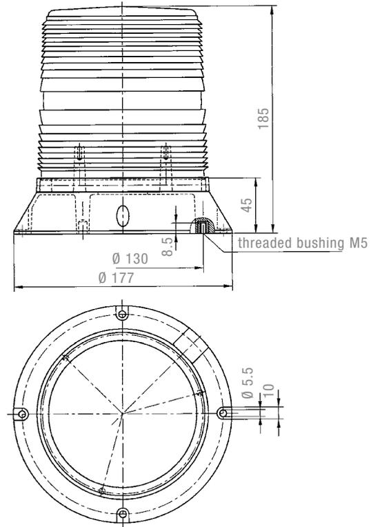
**Drilling template 1 for M5 threaded bushing**
