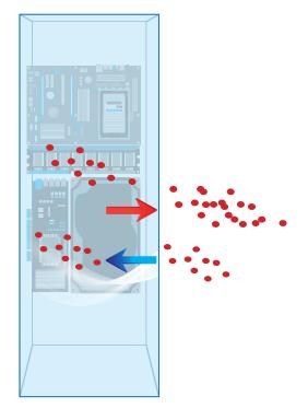
**Closed Loop Cooling**: Complete separation of internal and external air/water circuits **Open Loop Cooling**: Where ambient and internal air/water circuits mix
