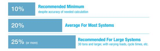
Derating the capacity can be a complicated calculation including the ambient environmental conditions, process temperature required, flow rate and size of lines, liquid medium, length/complexity of the plumbing from application to chiller and control requirements. These will all influence the end cooling result and can vary depending on the model of chiller selected for your application
